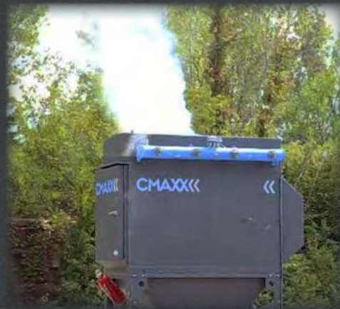
With cover on explosion vent, 100% of the flame front forced through the IDA DeltaMAXX Filters. No spark or flame present.
